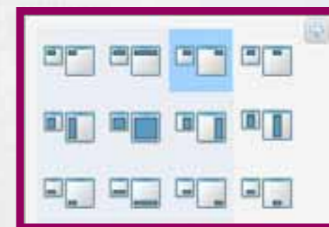
The Search control is defined with a top right anchoring, while keeping its size
