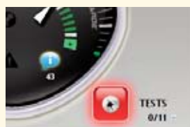
Excerpt from the dashboard: the red light indicates that the tests have failed or have not been run. Click to open the list
